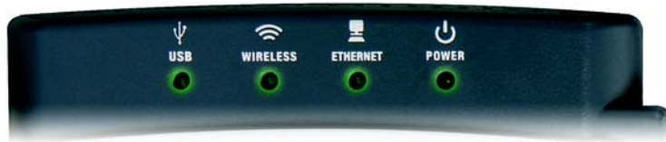
Figure 2-2: PrintServer's Front Panel
