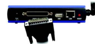
Figure 3-3: Connecting to the Parallel Port
