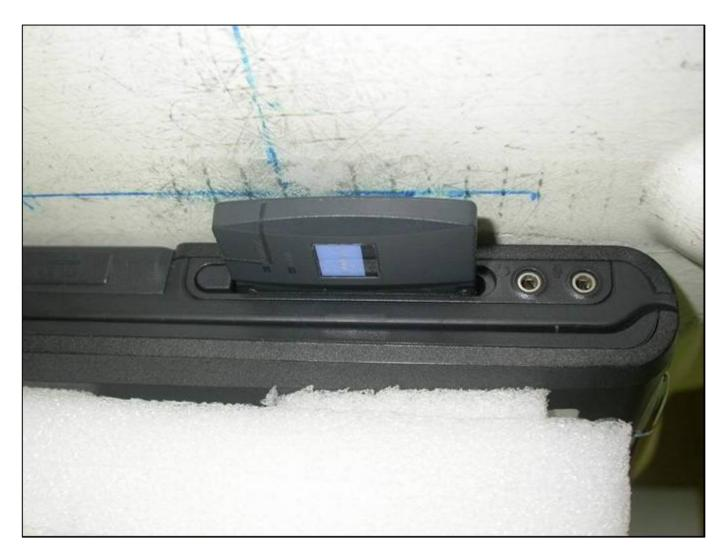
The bottom of the EUT to the flat phantom distance 11 mm
