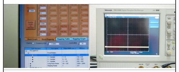
Radar 1 is used to test during DFS testing.
