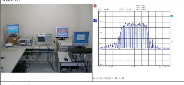
EUT (Client ) links with master on 5500MHz
