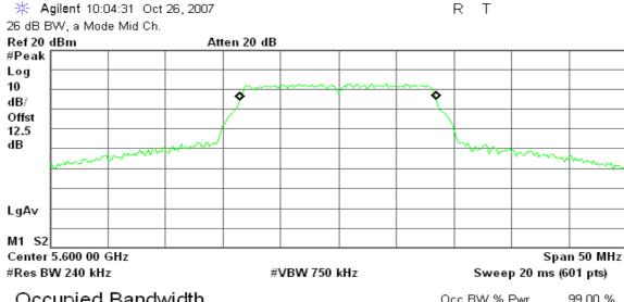
Occupied Bandwidth 16.9285 MHz Occ BW % Pwr 99.00 % x dB -26.00 dB
