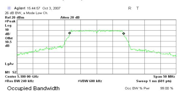
Transmit Freq Error 8.549 kHz x dB Bandwidth 20.241 MHz
