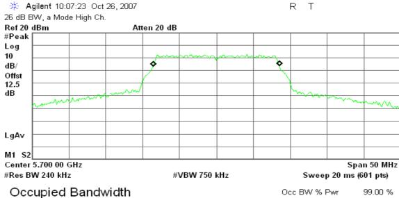
Occupied Bandwidth 17.0131 MHz Occ BW % Pwr 99.00 % x dB -26.00 dB
