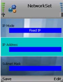
Figure 4-18: Network Settings - Fixed IP
