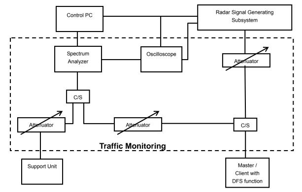
The test transmission will always be from the Master Device to the Client Device. While the Client device is set up to associate with the Master device and play the MPEG file ( $6\frac{1}{2}$  Magic Hours) from Master device, the designated MPEG test file and instructions are located at: <u>http://ntiacsd.ntia.doc.gov/dfs/</u>.
