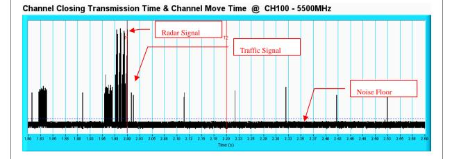
**NOTE:** An expanded plot for the device vacates the channel in the required 200ms.
