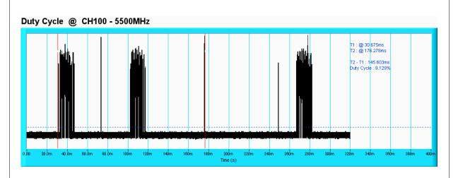
**NOTE:** T1 denotes the start of duty cycle period is  $0.030675^{\text{th}}$  second. T2 denotes the end of duty cycle period is  $0.17627^{\text{th}}$  second. T2 – T1= 0.145603 seconds. Duty Cycle = 9.129%
