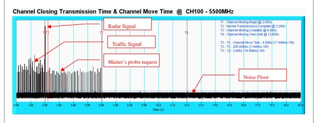
**NOTE:** T1 denotes the start of Channel Move Time upon the end of the last Radar burst. T2 denotes the data transmission time of 600ms from T1. T3 denotes the 10 second from T1 to observe the aggregate duration of transmissions.
