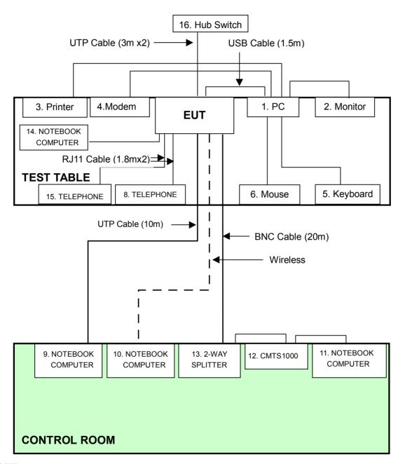
**NOTE:** 1. Support unit 9~13 were kept in the control room during the test.
