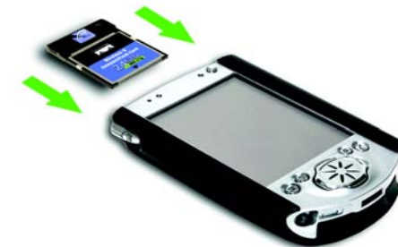
Figure 4-2: CompactFlash Installation into PDA
