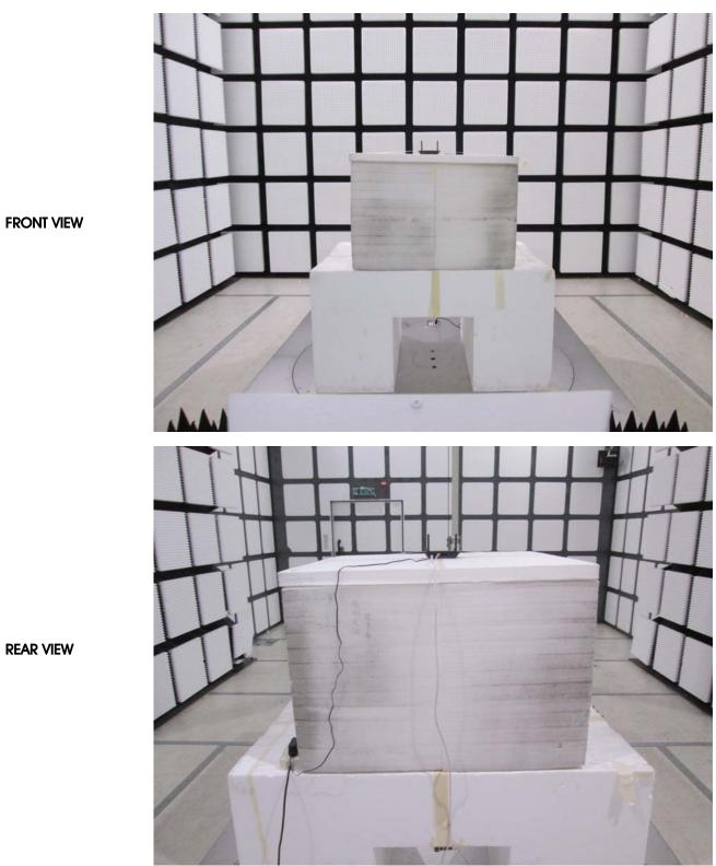
1. Photographs of Radiated Emissions Test Configuration
