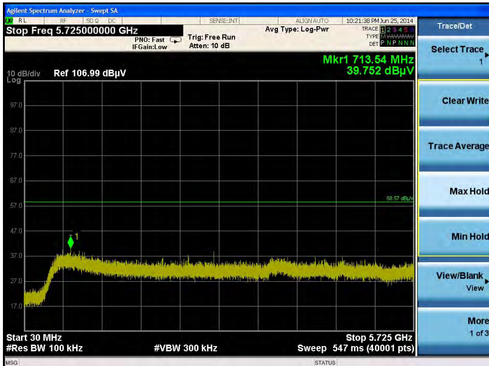
Plot on Configuration IEEE 802.11a / CH 165 / 30MHz~5725MHz (down 30dBc)
