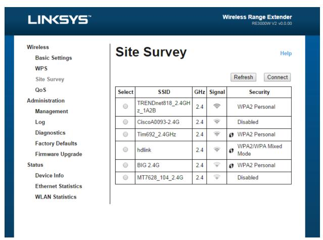
To connect your extender with an access point or router in Site Survey, you will need to know the password or passphrase of the network on that device.
