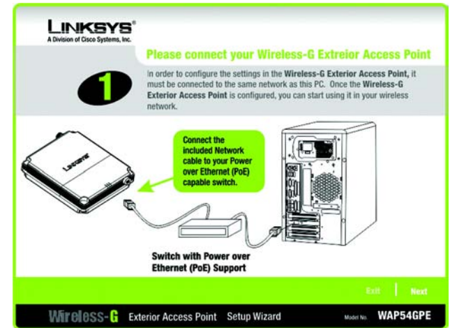
Figure 5-2: Connecting the Access Point
