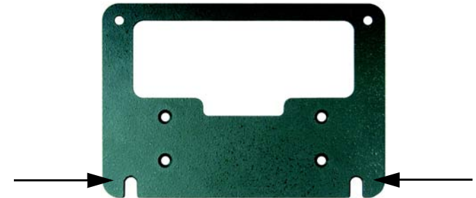
Figure 4-1: Mark the Locations of the Two Wall-Mount Slots
