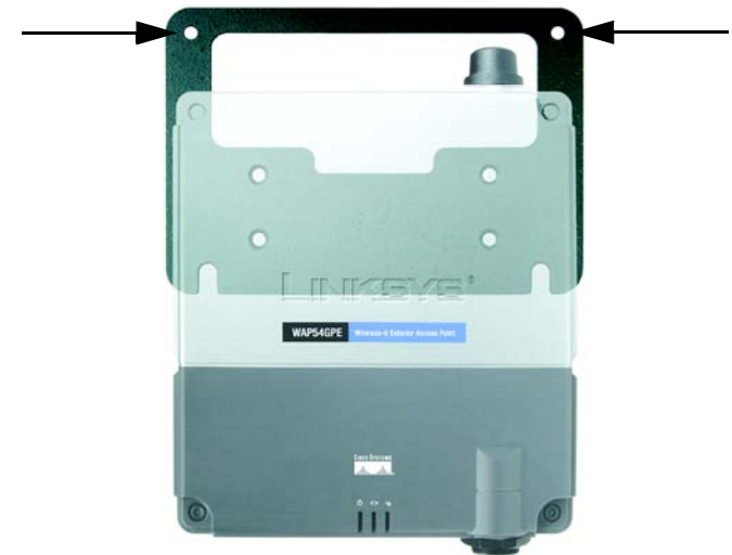
Figure 4-4: Attach the Access Point to the Wall
