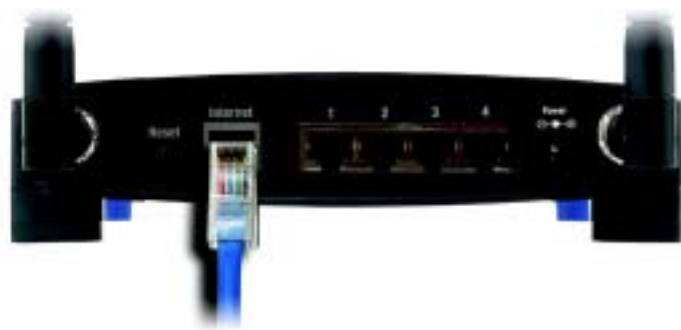
Figure 4-6: Connecting Another Router
