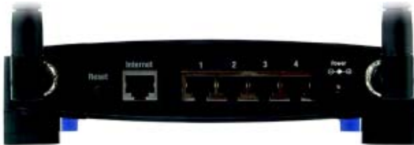
Figure 3-1: The Broadband Router's Back Panel
