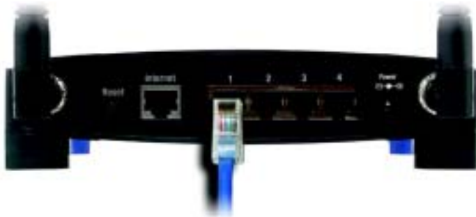
Figure 4-7: Connecting Your Network Devices
