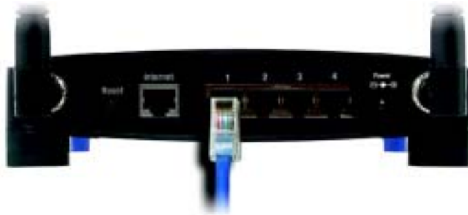
Figure 4-3: Connecting Your Network Devices
