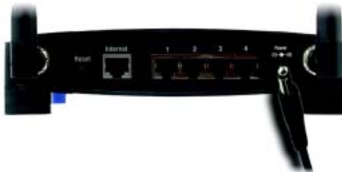
Figure 4-8: Connecting the Power
