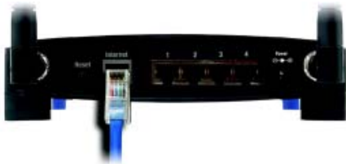
Figure 4-2: Connecting Your Internet Connection
