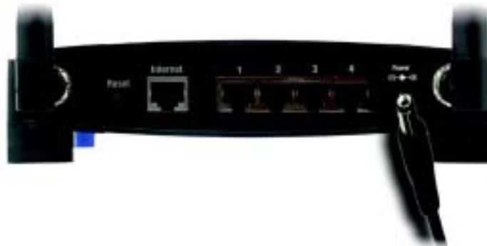
Figure 4-4: Connecting the Power
