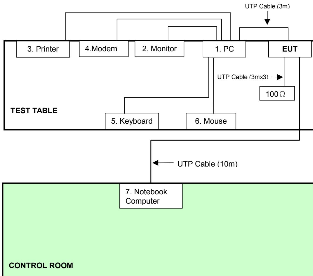
**NOTE:** 1. Support unit 7 was kept in the control room during the test.
