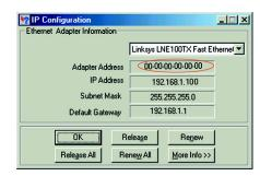
Figure D-2: MAC Address/Adapter Address
