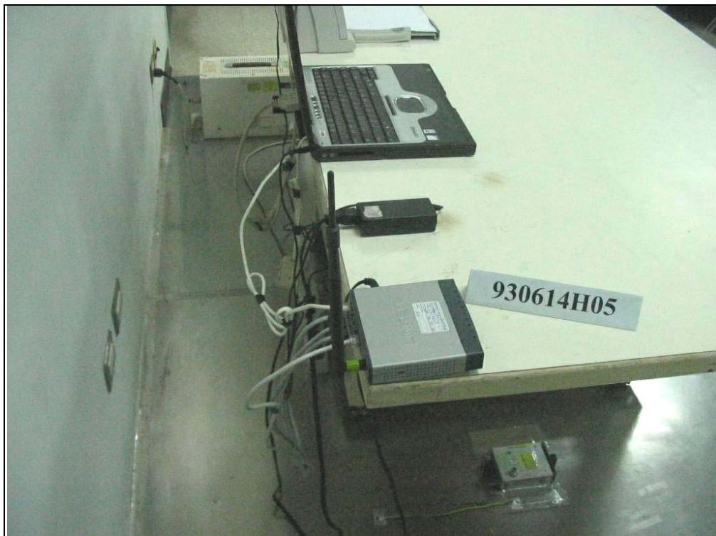
**RADIATED EMISSION TEST (antenna with the remote antenna-stand)**
