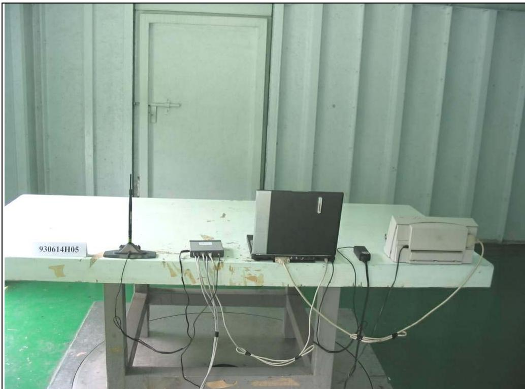
**RADIATED EMISSION TEST (antenna without the remote antenna-stand)**
