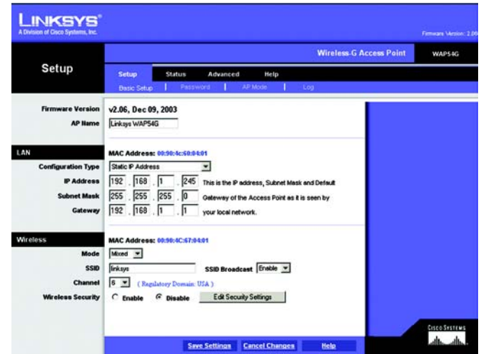
Figure 7-2: The Basic Setup Screen
