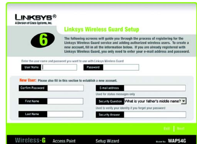
Figure 5-12: The Linksys Wireless Guard Setup Screen
