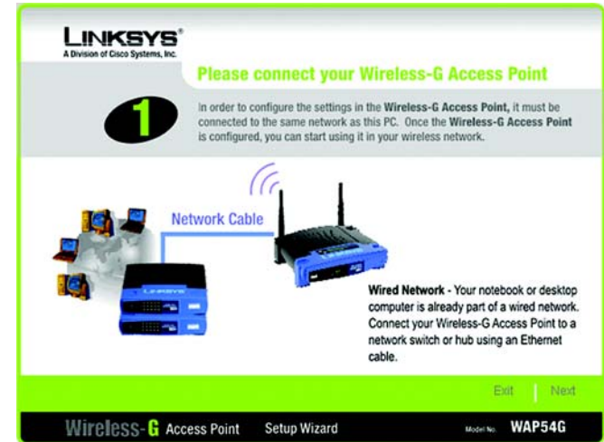
Figure 5-2: Connecting the Access Point
