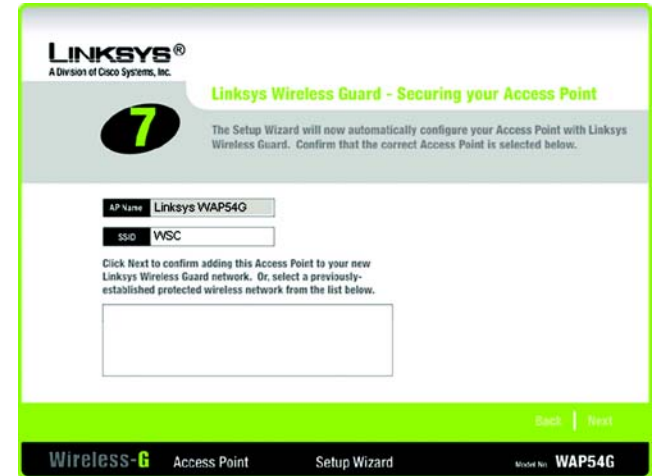
Figure 5-13: The Securing your Access Point Screen
