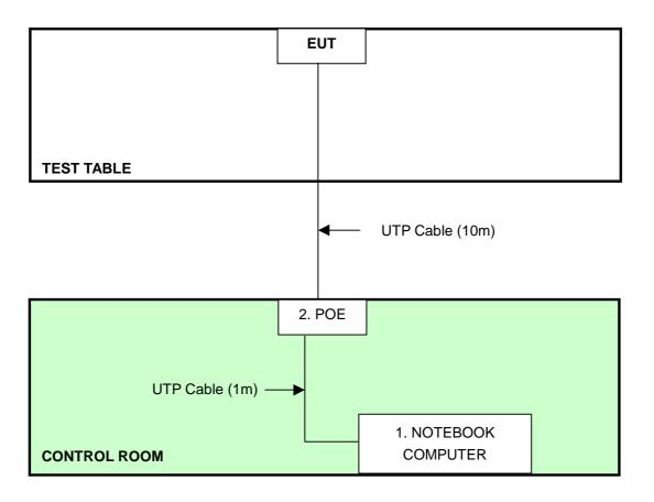
**NOTE:** 1. Support unit 1 and 2 were kept in the control room during the test.
