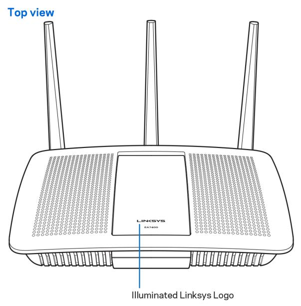
**Illuminated Linksys logo**—The Linksys logo stays on steadily while connected to the Internet. It flashes or pulses slowly during startup, self-testing and firmware upgrades. It flashes quickly when indicating connection errors.
