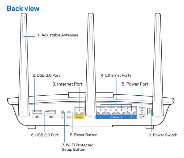
**Adjustable antennas (1)**—For best performance, position the antennas vertically as shown in the drawing.
