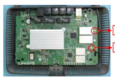
Chain 2 (Connect to Ant 2 for 2.4GHz/5GHz)
