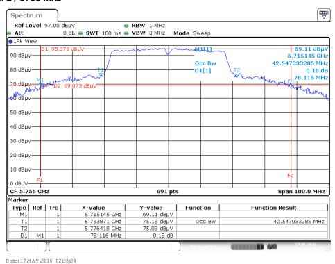
26dB Bandwidth and 99% Occupied Bandwidth Plot on Configuration IEEE 802.11ac MCS0/Nss1 VHT40 / Ant. 1 + Ant. 2 / 5795 MHz
