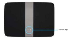
Indicator light—Stays on steadily while power is connected and following a successful Wi-Fi Protected Setup connection Pulses slowly during bootup, during firmware upgrades, and during a Wi-Fi Protected Setup connection Flashes quickly when there is a Wi-Fi Protected Setup error
