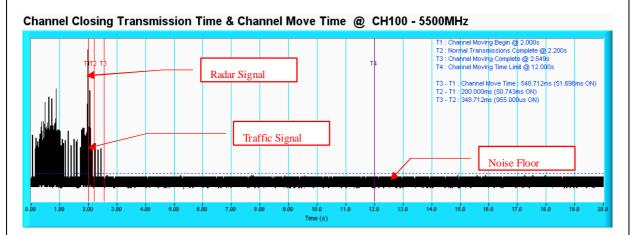
**NOTE:** T1 denotes the start of Channel Move Time upon the end of the last Radar burst. T2 denotes the data transmission time of 200ms from T1. T4 denotes the 10 second from T1 to observe the aggregate duration of transmissions.
