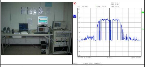
EUT (Client) links with master on 5500MHz
