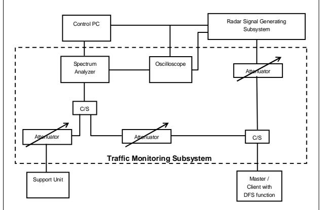
The test transmission will always be from the Master Device to the Client Device.
