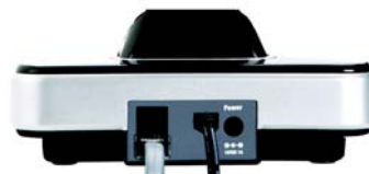
Figure 3-1: Telephone cable connection
