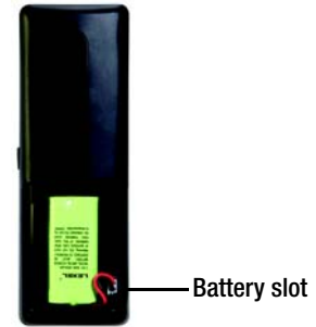
Figure 3-3: Battery pack installed
