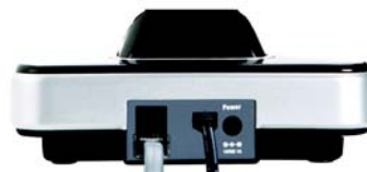
Figure 3-1: Telephone cable connection
