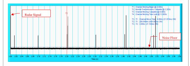
**NOTE:** A Zoom plot for the device vacates the channel in the required 600ms.
