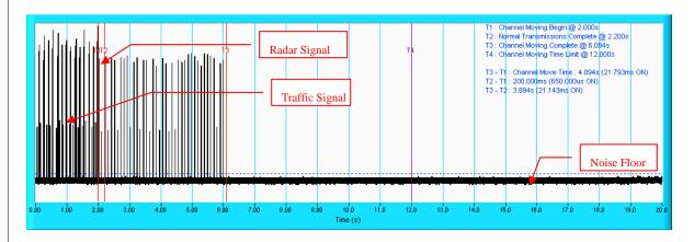
**NOTE:** T1 denotes the start of Channel Move Time upon the end of the last Radar burst. T2 denotes the data transmission time of 200ms from T1. T3 denotes the end of Channel Move Time.T4 denotes the 10 second from T1 to observe the aggregate duration of transmissions.
