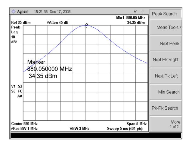
Down link Ch. 182. (Center channel) Cable loss = 0.4 dBRF Conducted power = 34.35 + 0.4 = 34.75 dBm \*
