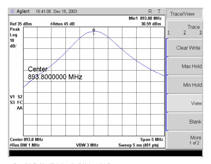
Down link Ch. 251. ( High channel ) Cable loss = 0.4 dBRF Conducted power = 30.59 + 0.4 = 30.99 dBm
