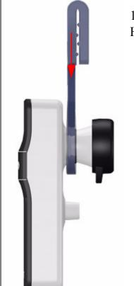
1. Push the headset clip onto the swivel at the back of the Voiis Headset.
