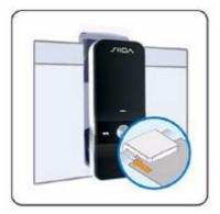
2. Clip the headset clip onto the rim of the collar or the shirt pocket, etc.
