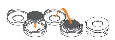
To charge your Q-70, place it in the charging box at the other end of the USB cable. Close the box afterwards, and make sure the Q-70 is securely covered. Plug the USB connector to either a PC or power adapter to start charging.
