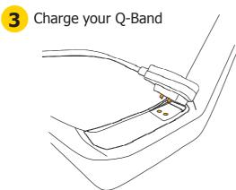
To charge your Q-Band, plug the charging cable into a USB port and attach the other end to the back of the Q-Band. A battery icon will appear on the screen displaying the charging progress. It takes around two hours to fully charge the battery.
