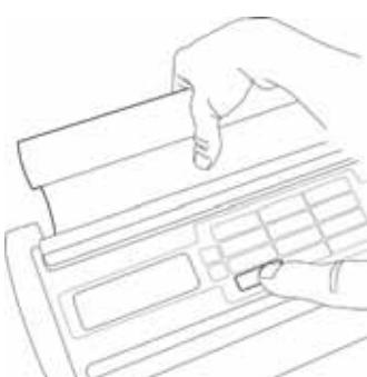
4. Insert paper in the paper slot and keep
