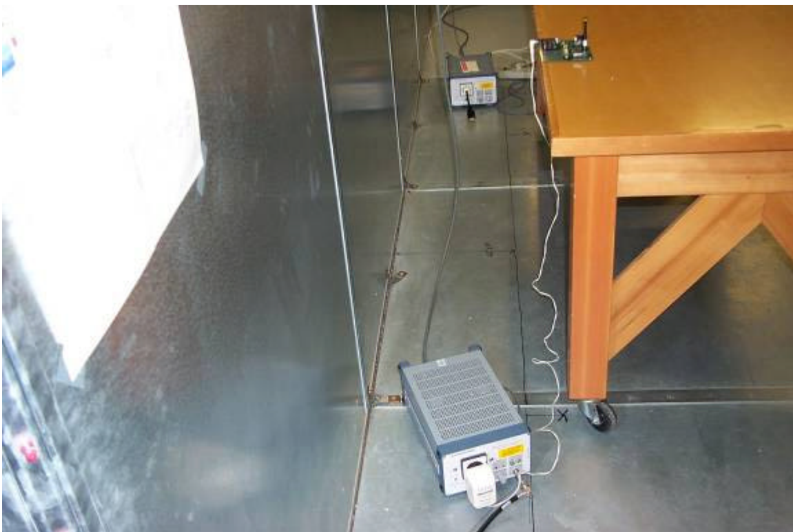
Figure 4 - Conducted Emissions Setup
