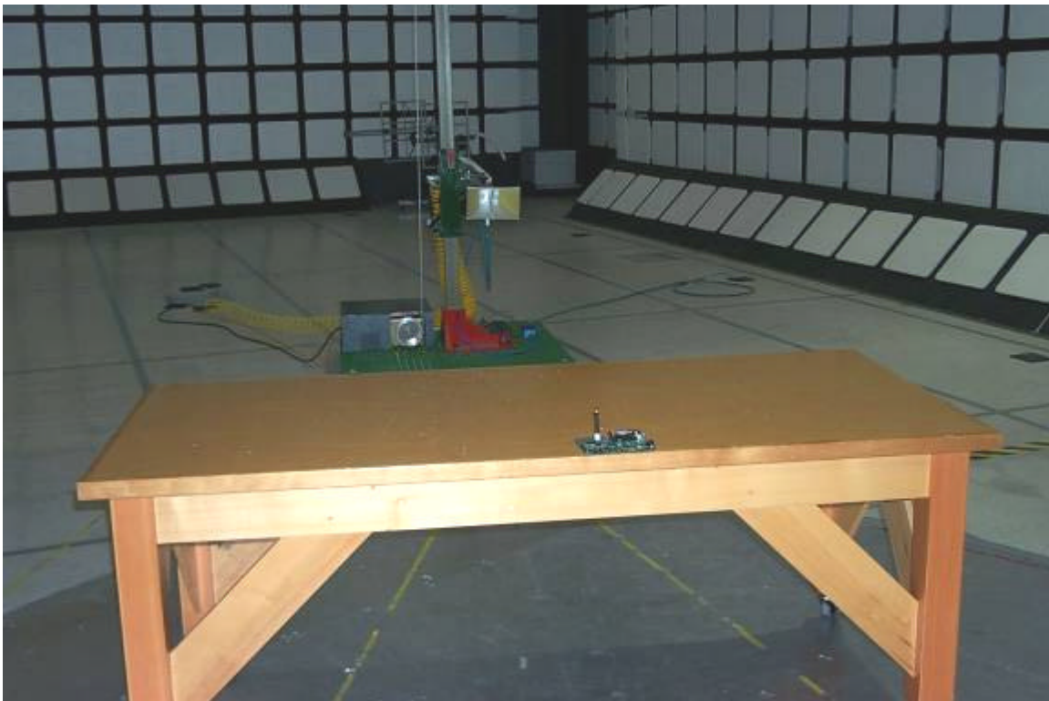
Figure 2 - Radiated Emissions Test Setup
