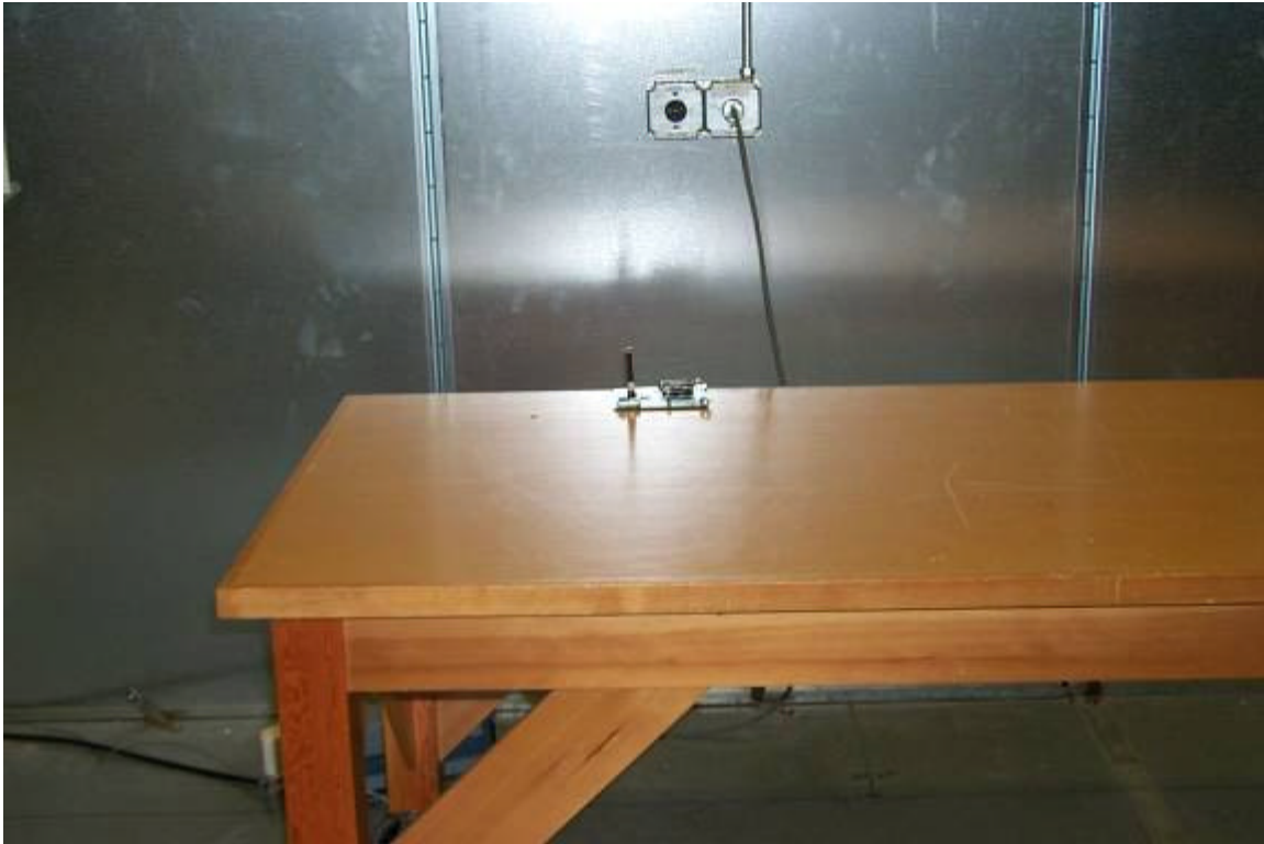
Figure 3 - Conducted Emissions Setup
