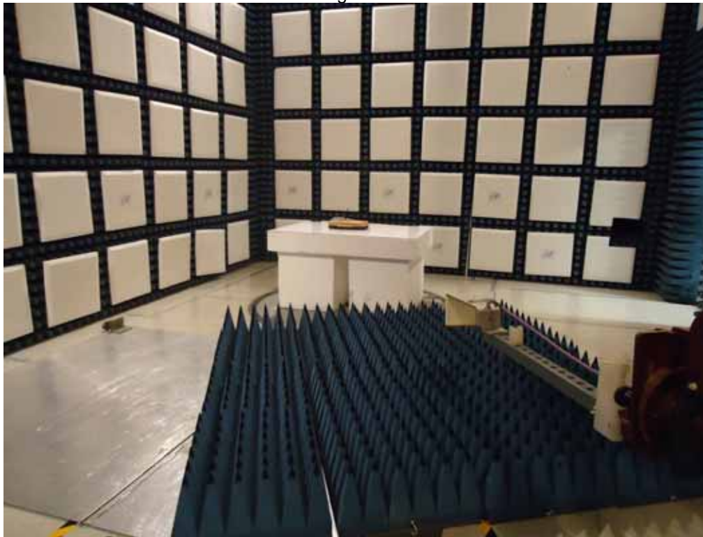
Test Setup for Radiated Emissions, Above 1GHz – Horizontal Polarization
