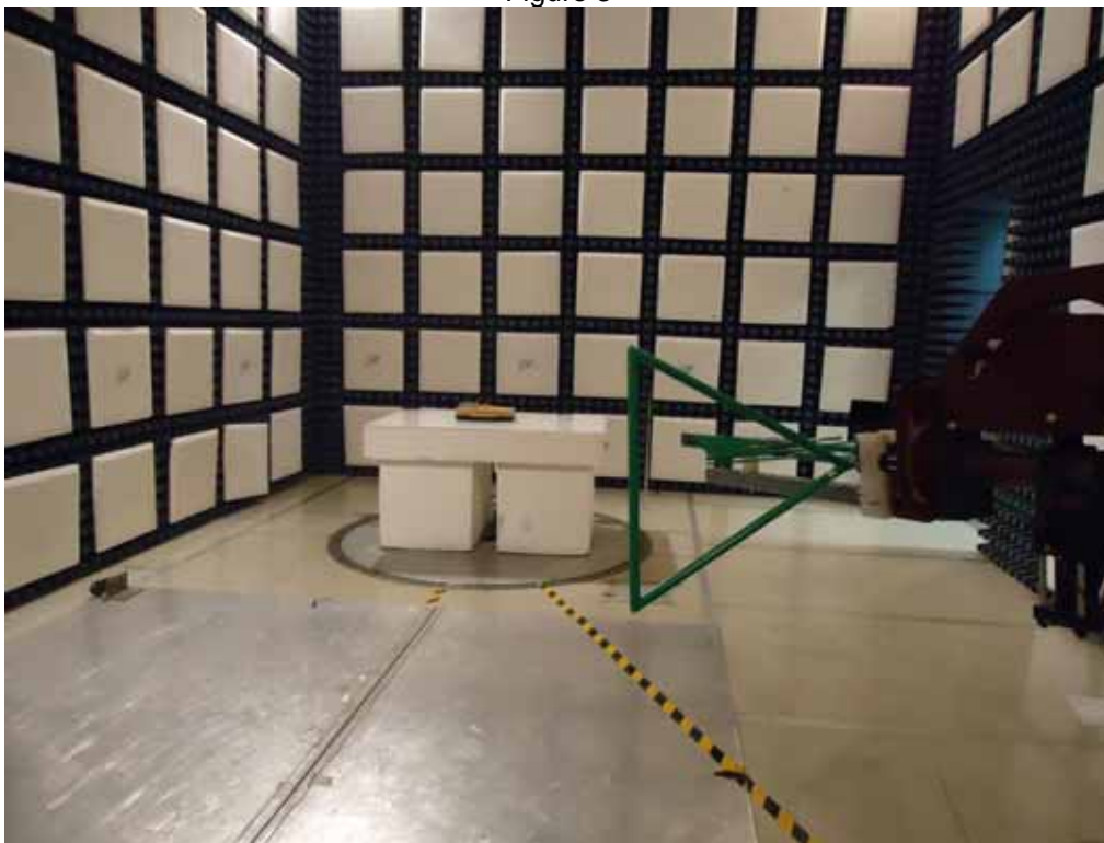
Test Setup for Radiated Emissions, 30MHz to 1GHz – Horizontal Polarization
