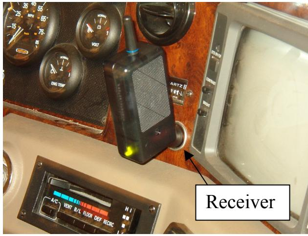
The Receiver plugs into a 12v outlet on the dash of the motorhome. When the BrakeBuddy is activated in the towed vehicle, the Receiver will illuminate.
