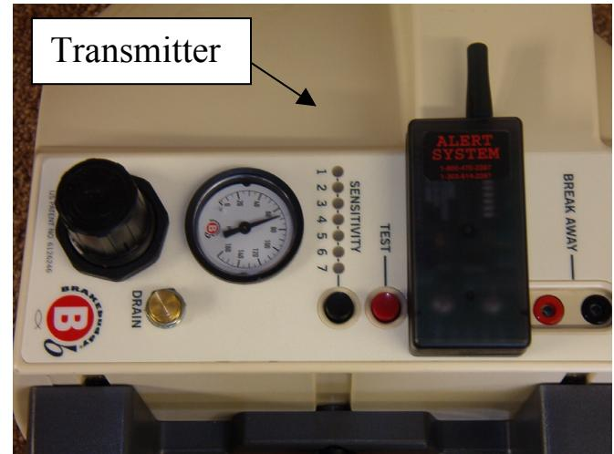
The Transmitter plugs into the top of the BrakeBuddy and sends a signal to the Receiver when the BrakeBuddy is activated.
