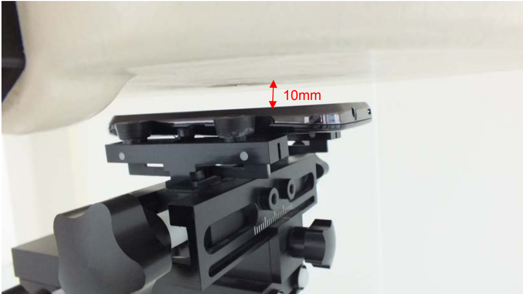
Picture 11: Back Side, the distance from handset to the bottom of the Phantom is 10mm
