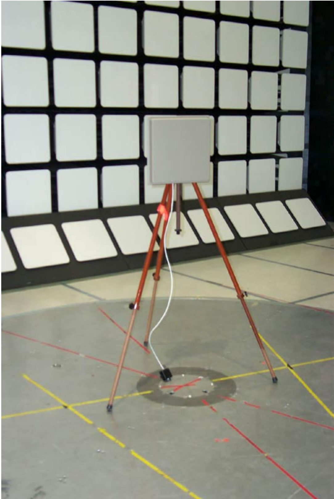
Figure 1 Radiated emissions test setup
