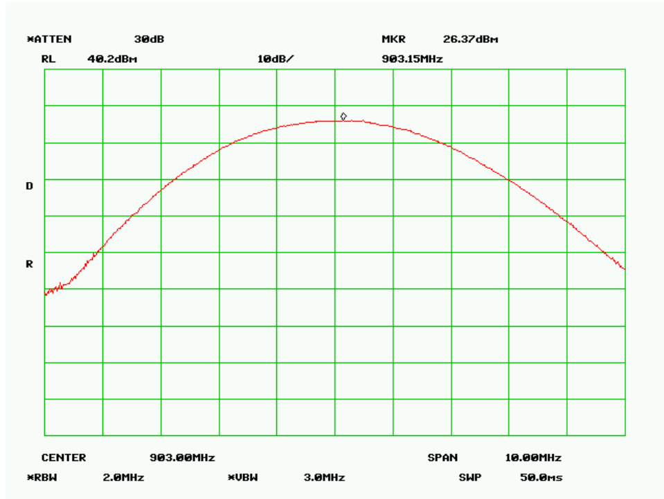
Output Power Low Channel (Antenna Gain 5dBi)
