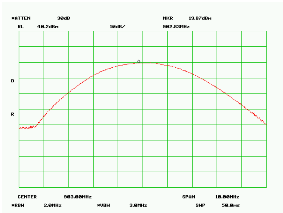
Output Power Low Channel (Antenna Gain 15dBi)
