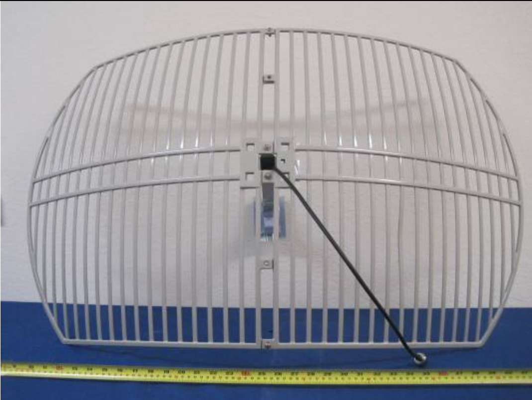
24dBi Gain Antenna – Back View
