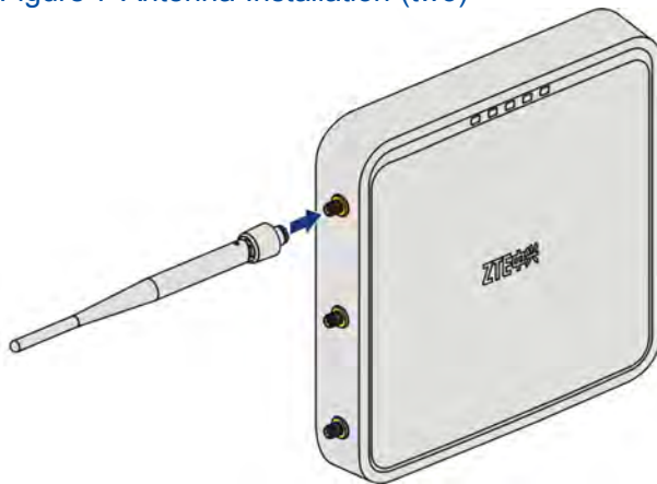
Figure 7 Antenna Installation (two)
