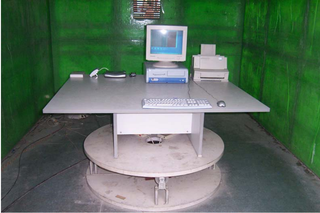
AC Power Antenna TDJ-2400BKF-Y: Radiated Emission - Front View
