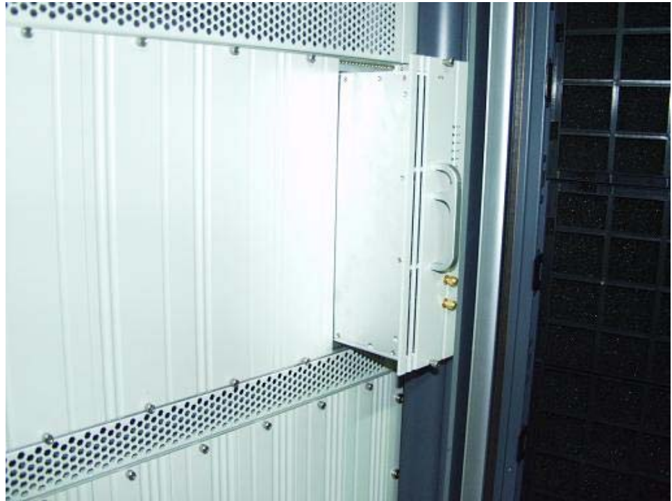
Fig. 12.3-3 Loosening the Screws and Unplugging the RFE
