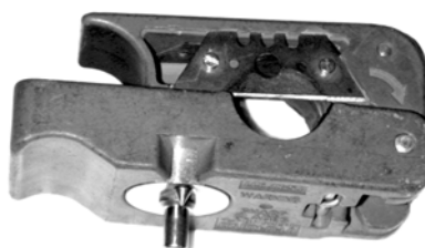
Fig. 10.4-6 Cutting Tool for the 7/8" Feeder Connector
