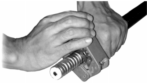
Fig. 10.4-7 Cutting the Feeder with a Cutter
