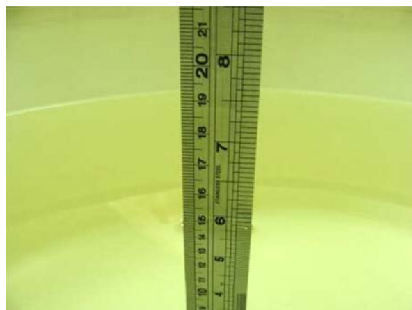
Fig 6.2 Photo of Liquid Height for Body SAR
