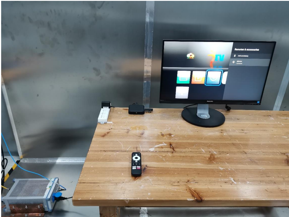
Photograph 3: Set-up photo for Conducted Emission
