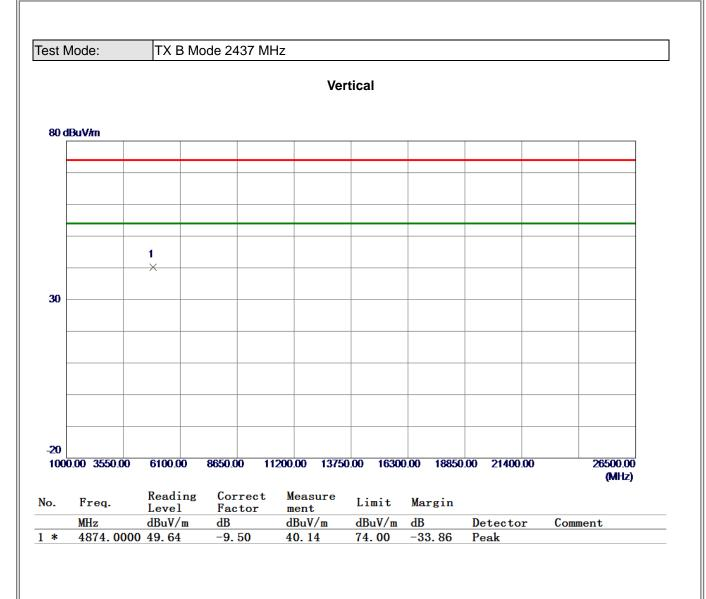
(1) Measurement Value = Reading Level + Correct Factor.
