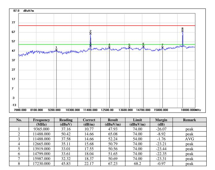
Note: 1. Measurement = Reading Level + Correct Factor.
