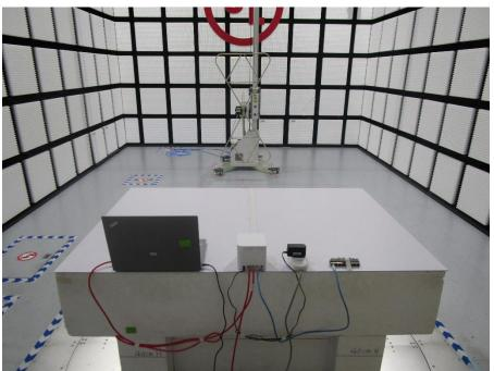
RADIATED RF MEASUREMENT SETUP (Below 30MHz)
