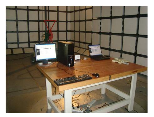
Radiated Emissions - Front View (Model: ZXDSL 831A [] with adapter 1)
