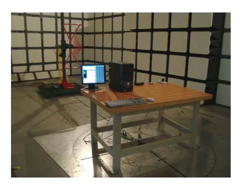
**Spurious Radiated Emissions - Rear View**
